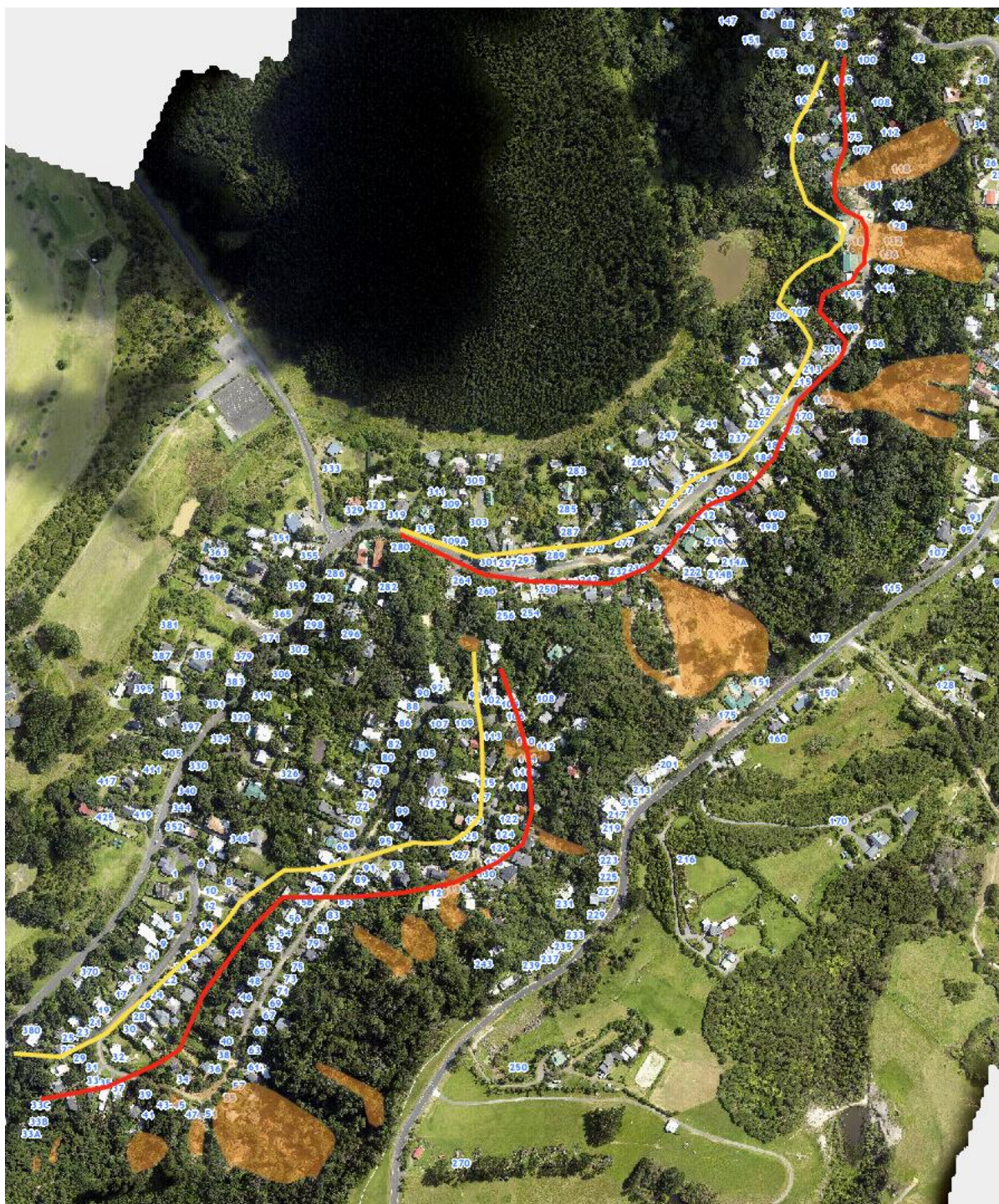
Figure 2 – Updated F-line assessment after on-site calibration. The red line shows the shortest likely landslide travel, and the yellow line shows the longest likely landslide travel. The orange areas are the landslide source areas.
