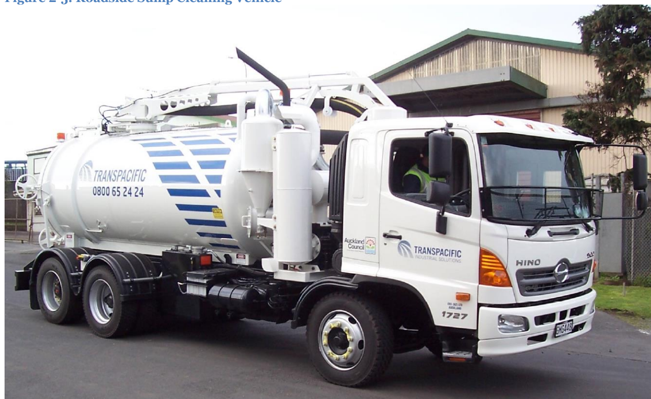
Figure 2-5: Roadside Sump Cleaning Vehicle
