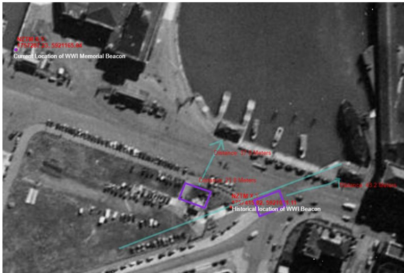
Figure 31. Historical 1940 aerial, with the original/ historical and current locations of the WWI Memorial Beacon labelled. The approximate original locations of ferry shelters is shown as purple rectangles and the distance (meters) given. The earlier sea wall alignment is indicated by the solid blue line (Auckland Council Geomaps)
