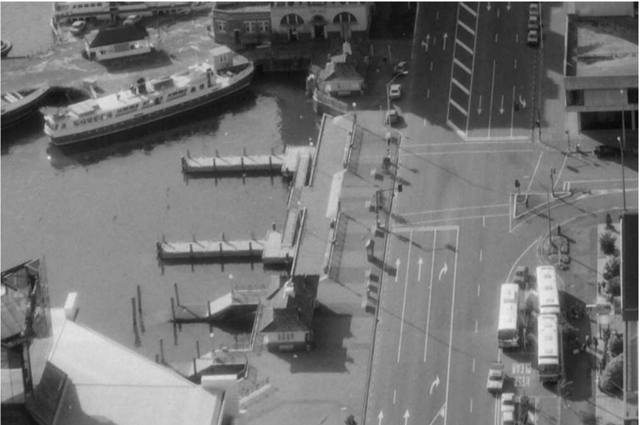
Figure 26. 1986 aerial photograph (and detail below) Princes Wharf and the Ferry Basin, showing 1980s deck extension, landscaping to the Ferry Basin and removal or obscuring of rail tracks/ tramlines (Alexander Turnbull Library WA-78938-F)
