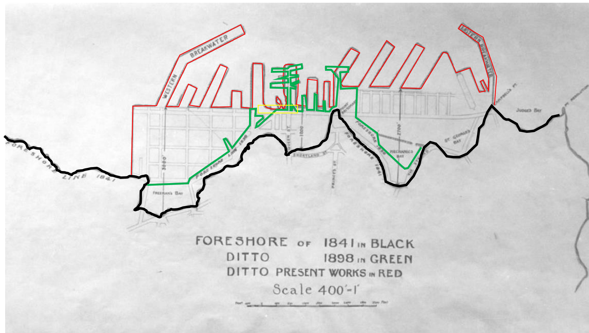
Figure 3. Map c. 1910-1920; showing progressive reclamations of the Auckland foreshore with approximate location of the Quay Street Enhancements Project shown in yellow (Auckland Libraries Special collections 4-8477)
